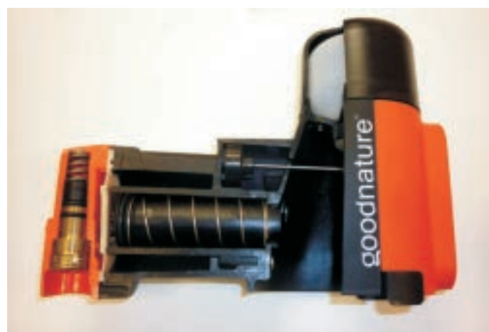
Cut-away of the A24 automatic killing device for rats and stoats. The NZ government is currently conducting a three year field trial to assess their suitability
